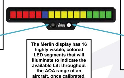
Brightness button when depressed repeatedly will increase the light level through 16 steps until its maximum then drops to the minimum level and steps up each time the button is depressed.
